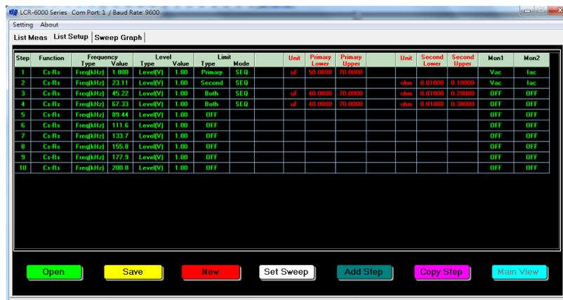
Function: Click on the Function icon to choose the primary and secondary measurement parameters in the pull down menu.
