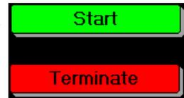
Terminate: Click on the Terminate icon to stop a sweep test.
