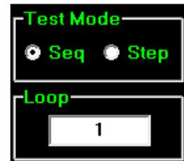
Loop: Loop is used to set the maximum sweep count for all the listed steps; the maximum settable value is 1000.
