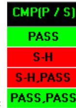
PASS: The measured value falls inside the tolerance range.
