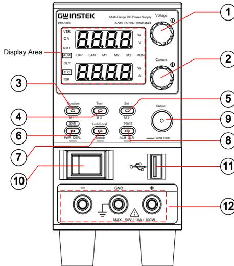
**Display Area** The display area shows setting values, output values and parameter settings. The function LEDs below show the current status and mode of the power supply. See page 16 for details.
